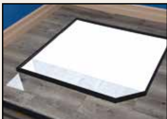
9. Lay in (1) 6" x 36" Cement Board rectangle piece with two end cuts.
